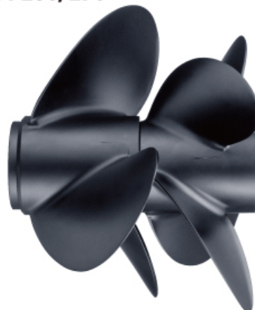
Aluminum / 3 blade front & 4 blade rear / Rubber hub
